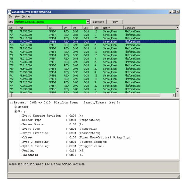
Running the UTC001 as the protocol analyzer allows monitoring, injecting, capturing and validating I<sup>2</sup>C traffic on any of the Intelligent Platform Management Busses (IPMB). A Graphical User Interface (GUI) validates and displays the IPMI packets or schedules IPMI messages for injection into the system. The GUI application communicates with the integrated UTC001 IPMI controller through an Ethernet port.
