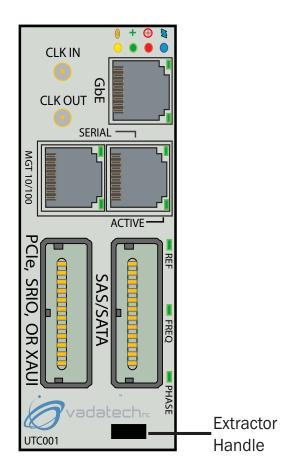
FIGURE 2. UTC001 Front Panel Diagram
