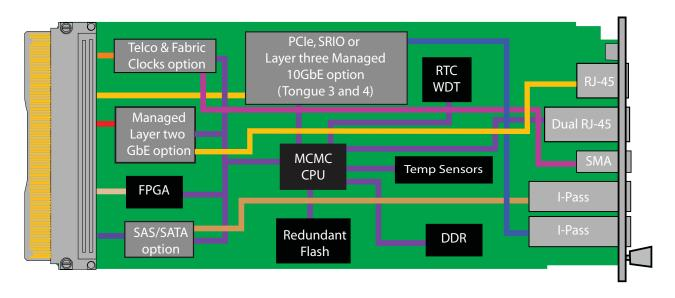
FIGURE 1. UTC001 Functional Block Diagram
